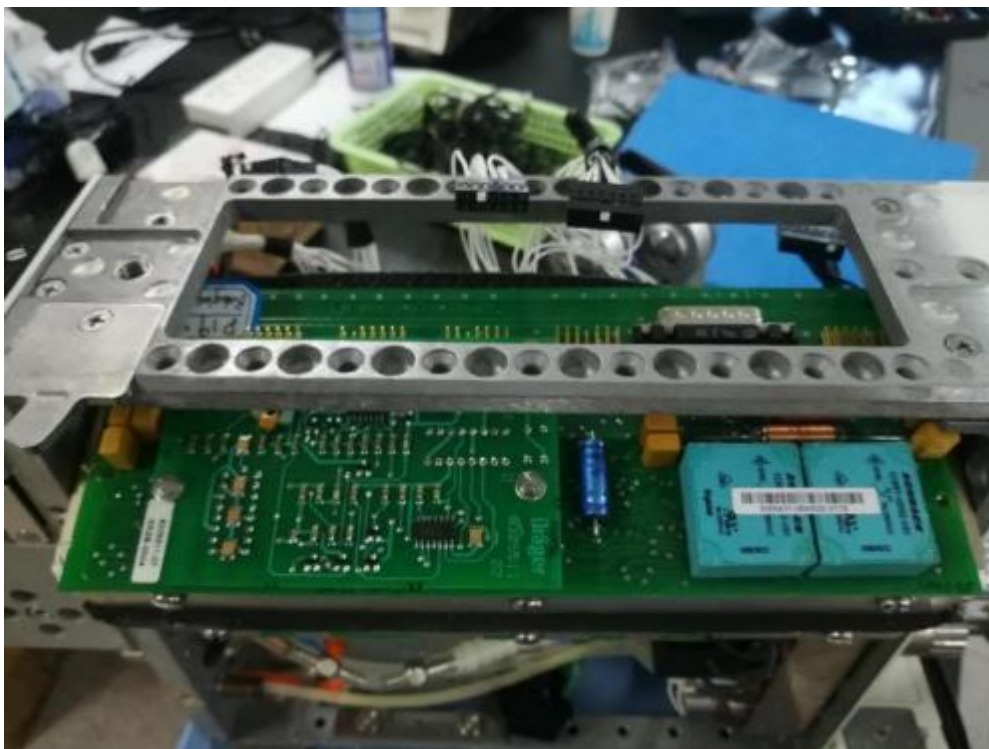
Figure 7: Valve Control Board
