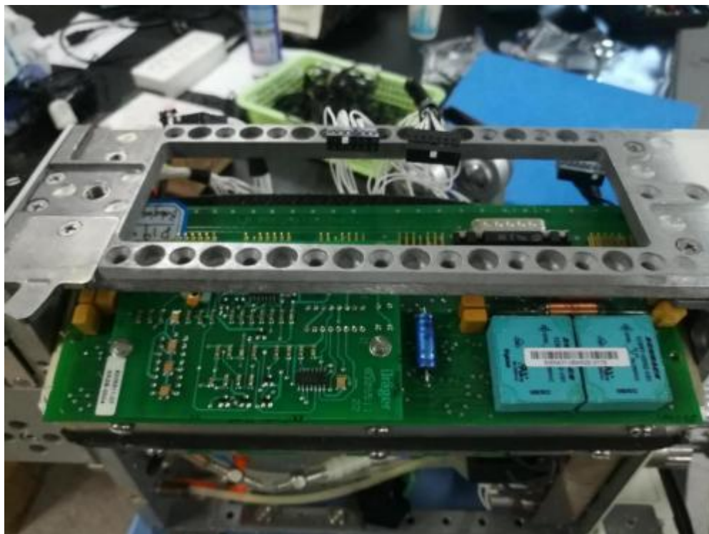
Figure 7: Valve Control Board
